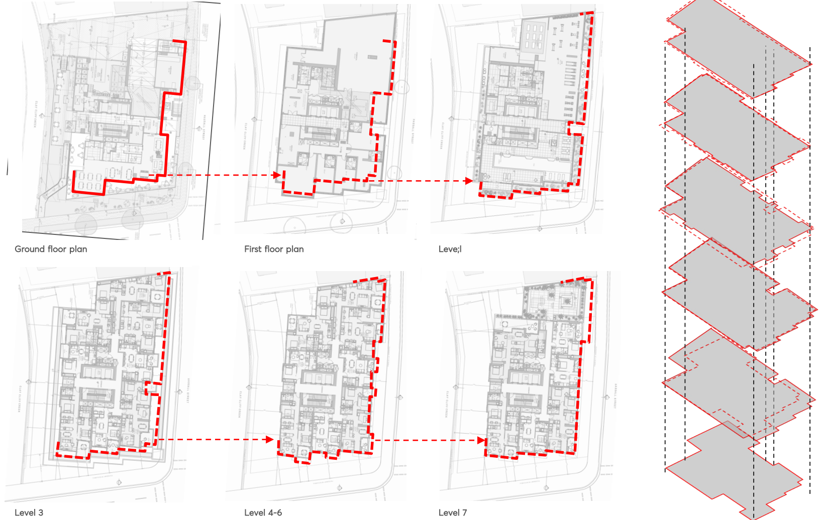
PODIUM FLOORPLATES OVERLAYED ON EACH OTHER IN PLAN AND ISOMETRIC VIEW, RESULTING IN AN INCONSISTENT STREET WALL
