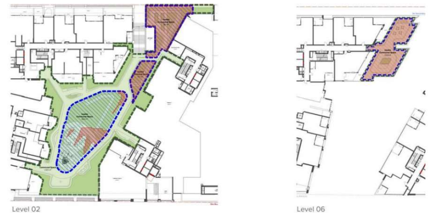
Figure 28 | Communal open space solar analysis (blue represents the principle useable open space, red illustrates the areas receiving two hours of solar access) (Source: Applicant's Additional Information)
