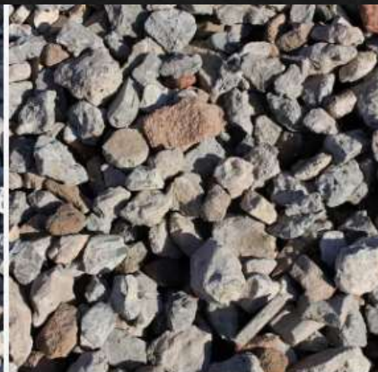
Oversize Crushed Concrete Aggregate
