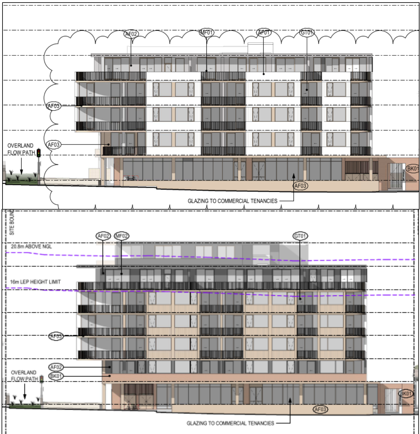
Figure 20 | Building A, Delmar Parade approved DA (top) and proposed (bottom) podium height comparison
