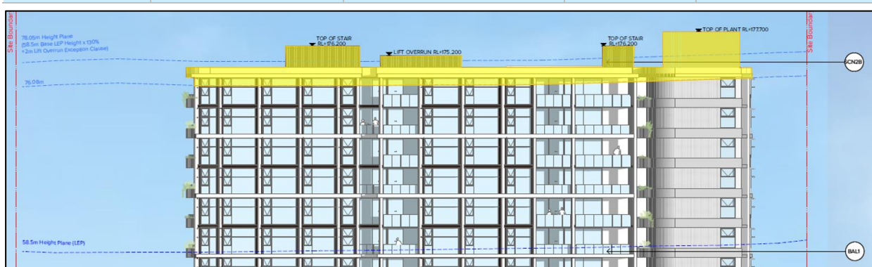
Figure 8 | Extract of Alexander Street elevation with extent of height breach highlighted in yellow (Source: Applicant’s additional information)
