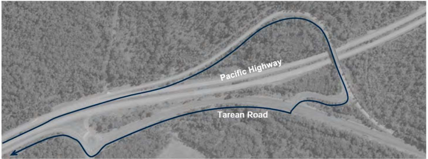
Figure 6-10 Proposed U-turn movement at Tarean Road interchange
