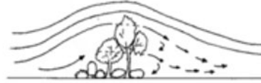
Fig. 2. With a permeable windbreak winds are slowed as they pass through the windbreak so the pressure difference in the lee is less pronounced compared to a solid barrier & so turbulence is greatly reduced.
