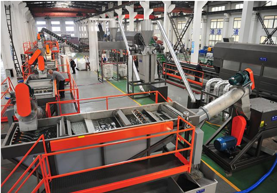
Figure B 1 - Example of PET bottle washing and waste lines (Beier Machinery) Figure A.9 provided in the EIS by GHD (2022). Note that there are no ventilation hoods, ducting or filters provided to prevent exposure to airborne particulate generated by the waste plastic handling and shredding processes and the many toxic chemicals and hazardous materials in and generated by contaminated waste. The rotating machinery within each open topped tank is unguarded and there is no evidence of electronic guarding.
