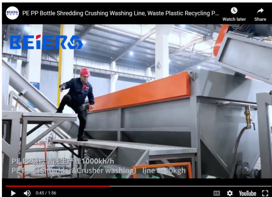
Figure B 6 - Visible airborne particulate and lack of handrails and stairs.
