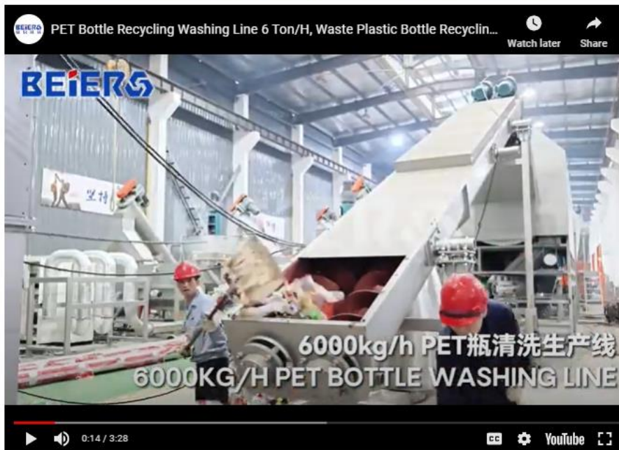
Figure B 14- Shovel-feeding from floor, lack of guarding around exposed operating augers, and hitting and risking cutting of the overhead wire with the sharp edge of the shovel.
