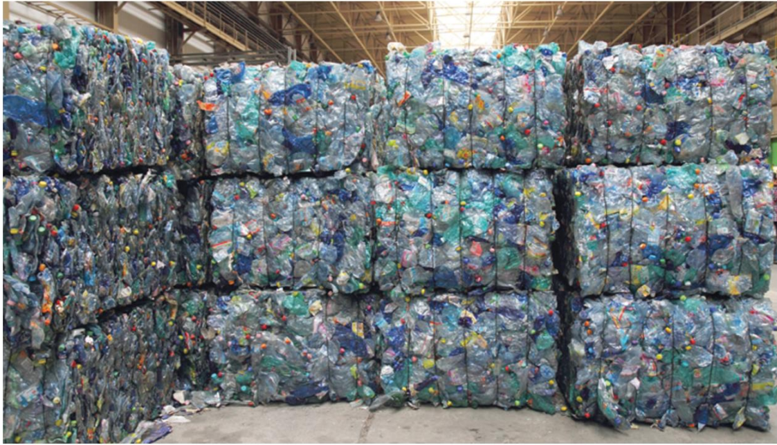
Figure 6 - Baled plastic bottles as stored at Plastic Revolutions Inc. is a recycler in Reidsville, North Carolina, that takes in scrap plastics and granulates and washes, pelletizes expected to be similar to the proposed facility. https://www.recyclingtoday.com/article/plastic-revolutions-plastics-sorting-baling/
