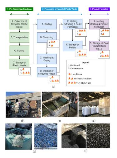
commercial plastic recycling facilities, <u>https://doi.org/10.1177/073490412311998</u>) which indicates both the likelihood and consequence of a fire in the different stages of the recycling process.
