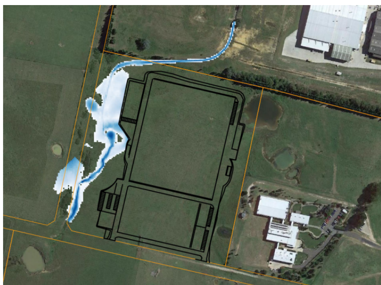
Figure 3. Design Flood Extent, Moss Vale Plastics Recycling and Reprocessing Facility. Technical Report 10 - Soils and Water. Plasrefine Recycling Pty Ltd. 22 December 2021. Figure 3.3, p.13 [ref 75]
