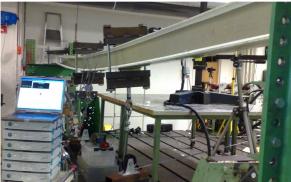
Figure 7 Photo: Bending test of a section on a wing profile. Own photo, from testing
