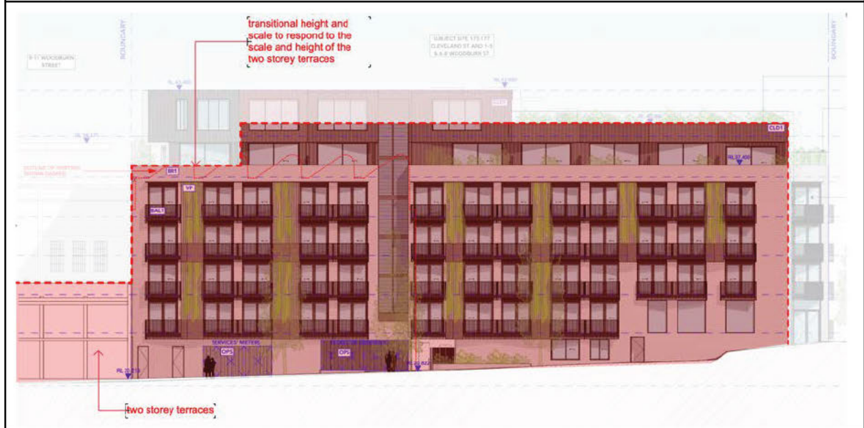
Figure 32: Excerpt of SSD2401 East Elevation (Woodburn Street) showing different options for a transitional scale that would be more appropriate to the adjacent height, bulk and scale, creating a more harmonious streetscape and would largely remove the amenity issues.
