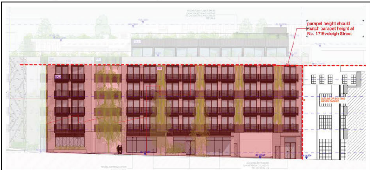
Figure 29: Excerpt of SSD2400 West Elevation (Eveleigh Street) – the proposed street parapet should match the existing parapet height at No. 17 Eveleigh Street.
