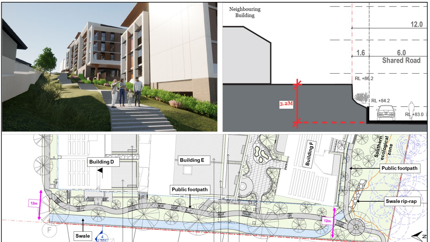
Figure 18 | Perspective looking north along the western setback footpath (top left), section indicating excavation necessary to construct a road (top right) and proposed western setback layout (bottom) (Base source: Applicant's RtS and RRFI)
