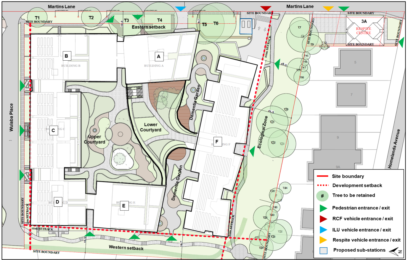
Figure 12 | Proposed building layout, setbacks, vehicle, pedestrian entrances and trees and open spaces (Base source: Rts)
