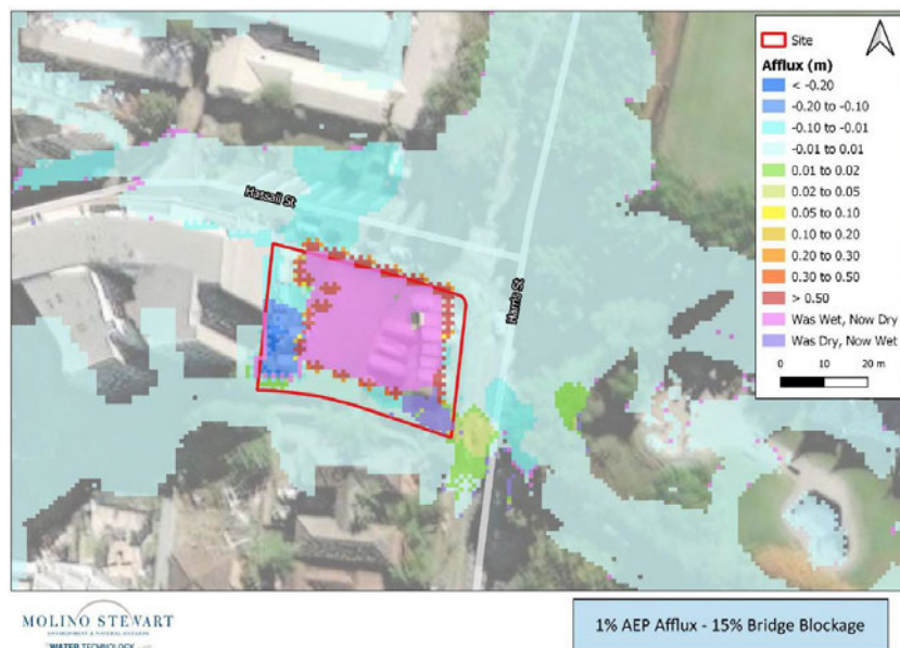
Figure 3: Flood Level Difference (Proposed minus Existing case) – 1% AEP Design Event including 15% Bridge Blockage
