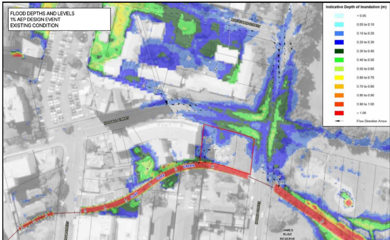
Figure 6 – Flood Depths and Levels – 1% AEP Existing Conditions (Lyall & Associates, 2022)
