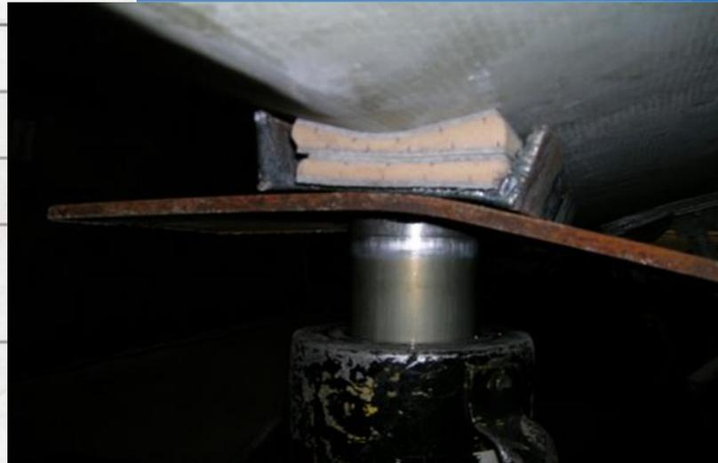
This picture is of two, one (1) inch panel sections of composites material supporting a 168,000 lbs vessel. Notice that the load is absorbed in only one of the top panel's two structural skins. The 1/2" steel plate bent under the load
