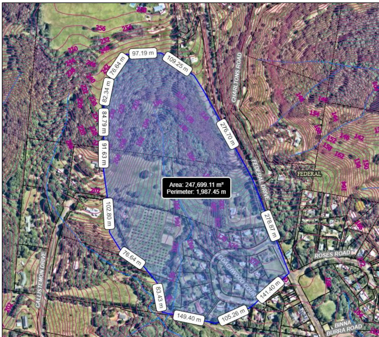
Figure 3. Catchment area of the pond
