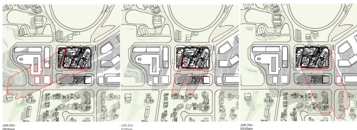
Figure 24 | Overshadowing impacts on surrounding developments, 21 June (Source: RtS)
