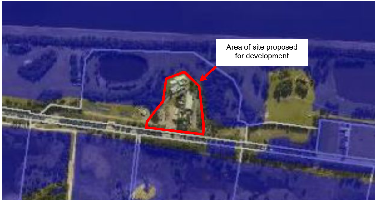
Figure 7 | Area of site proposed for development with 0.2% AEP flood extent shaded purple (Source: Applicant's Floodplain Risk Management Assessment)
