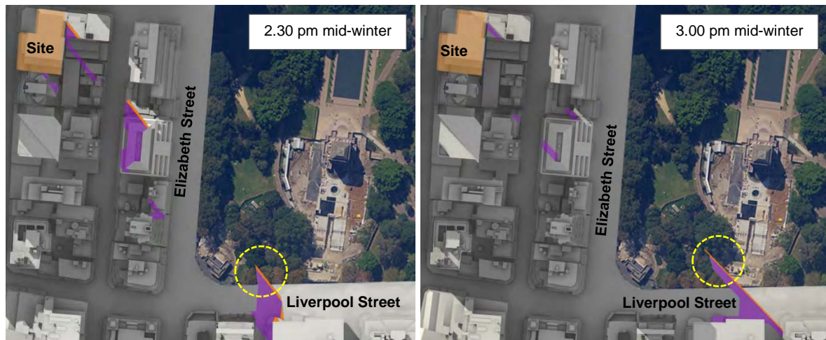
Figure 23 | Midwinter shadowing impacts of proposal shown in purple. Shadow impacts of approved building envelope shown orange (Base source: RTS)
