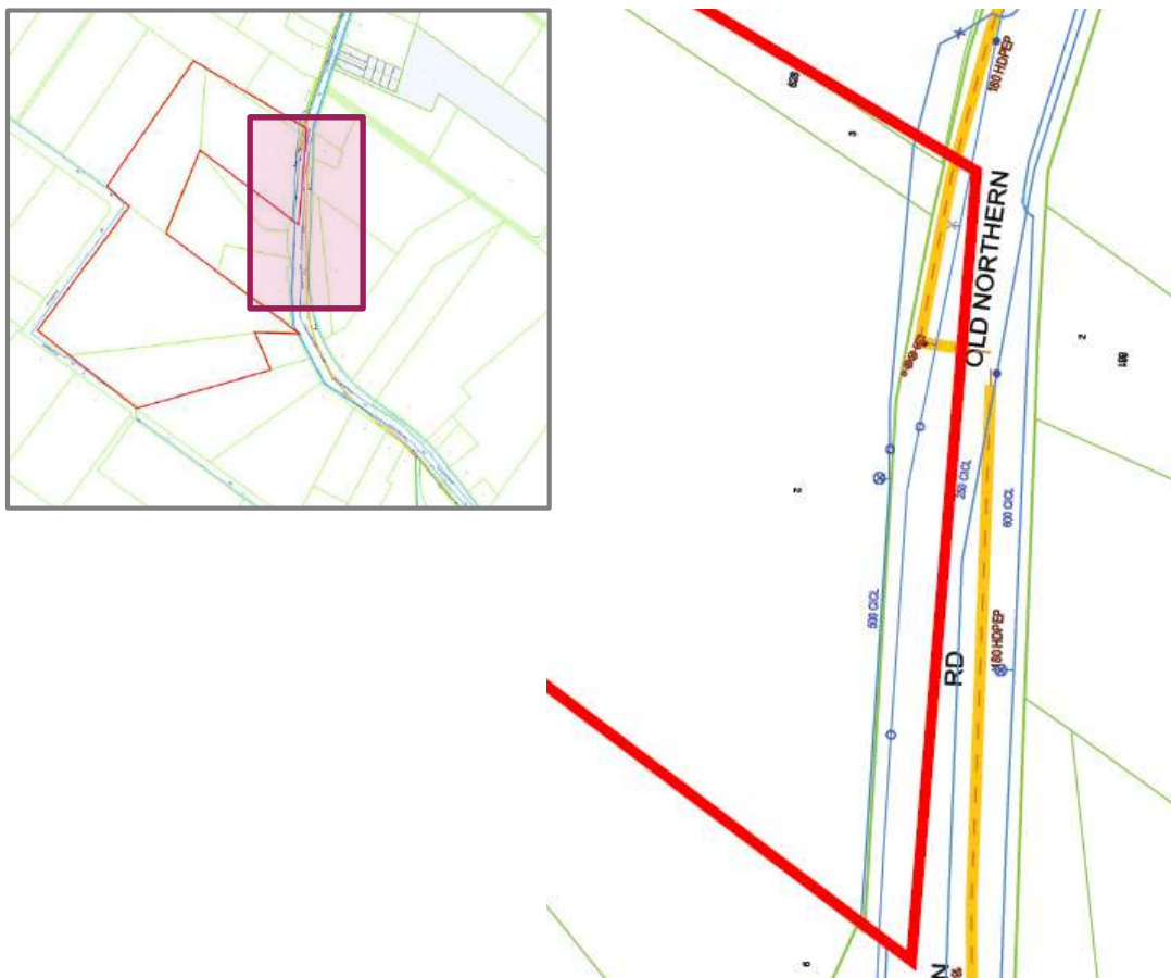
Figure 1. Extract from DBYD records illustrating the water mains (shown in blue) and the newly constructed rising main (shown in orange) with reference to the northern site boundary (shown in red)
