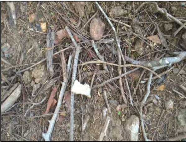
Photograph 2 – Presumed asbestos fibre cement debris on the western boundary.
