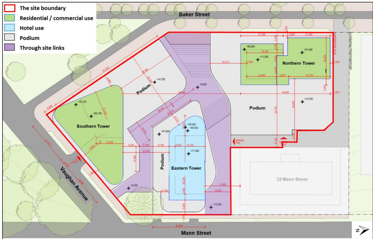
Figure 12 | The concept proposal layout and location of uses (Base source: Applicant's RtS)
