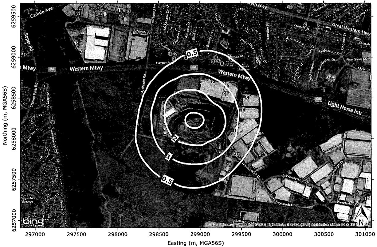
Figure 7 | Modification Increment Annual Average PM<sub>2.5</sub> Concentration (µg/m<sup>3</sup>) (AQIA 2018)
