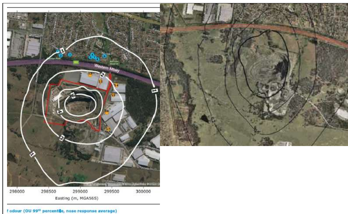
Figure 3-5. AQIA, 1-hour 2 ou, 99.5% odour concentration footprint (left) v.s. original EIS, 1-hour 2 ou 99.5% odour concentration footprint (right).
