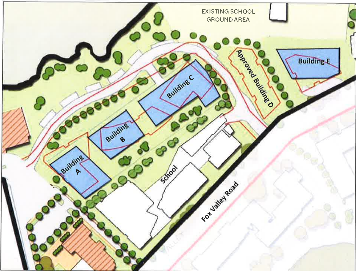
Figure 7 | Proposed building footprints and road alignment shown coloured compared to approved footprints and road alignment shown outlined in red (Base source: SRTS)
