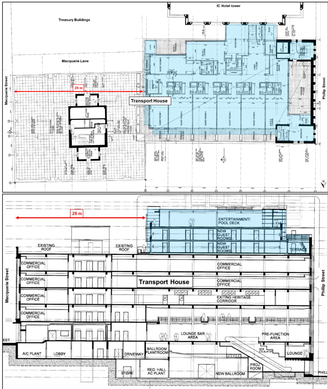
Figure 8 – Original Approval for 3 storey Transport House roof addition layout (top) and section (bottom) highlighted in blue and the approved setback from Macquarie Street (Base source: the Original Approval)
