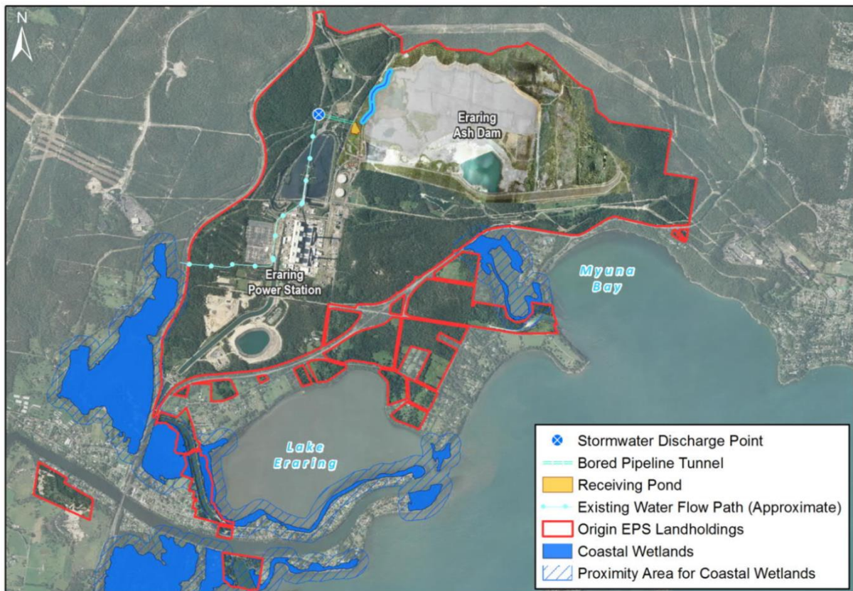
Figure 11 | Proposed stormwater flow path and discharge point
