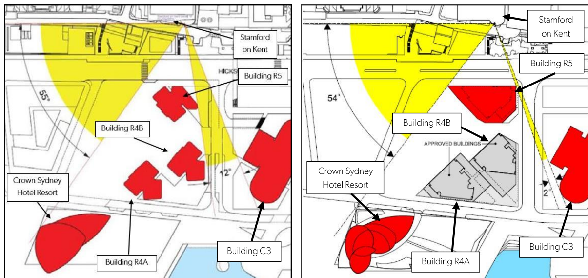
Figure 19 | Stamford on Kent example of view angle calculation of indicative (left) and approved maximum (right) Concept Plan building envelopes (Base Source: Applicant's VVIA)
