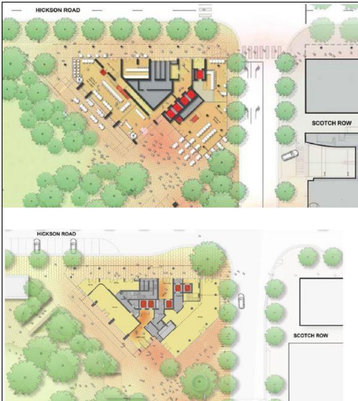
Figure 11 | Relationship between podium and Scotch Row – exhibited (top) and RtS (bottom) (Source: RtS)
