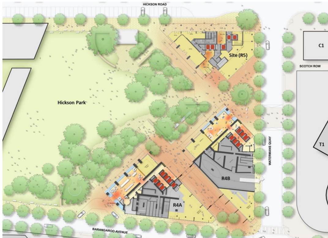
Figure 4 – Ground floor plan of the tower and its relationship to existing and proposed neighbouring buildings and spaces (Base source: Applicant’s Supplementary Design Report)
