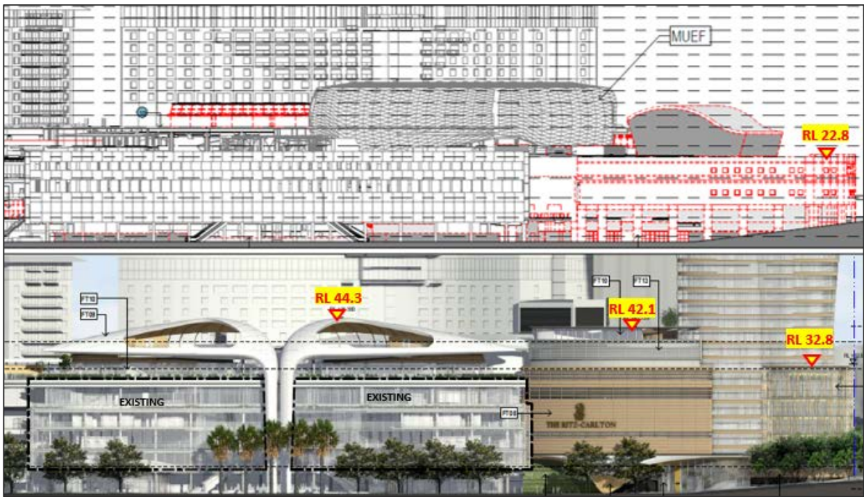
Figure 15 Existing (above) and proposed Pirrama Road podium elevation (note: red dashed line denotes demolition) (Base source: Proponent's Architectural drawings)
