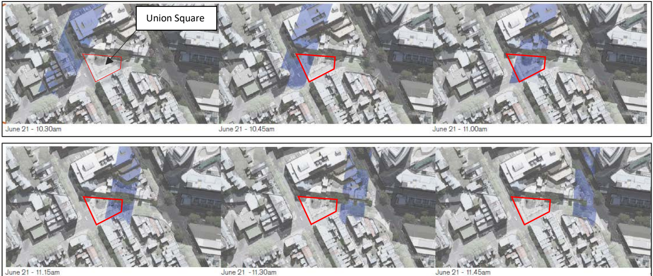
Figure 36 | Shadow diagrams indicating peak day overshadowing (blue) of Union Square (red) (Base source: Proponent's RtS)
