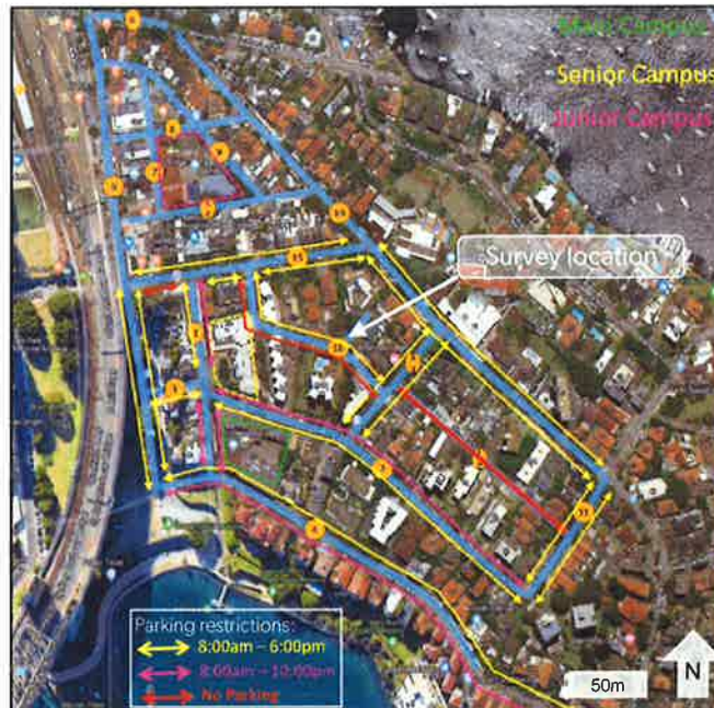
Figure 49 | On street parking demand survey locations and parking restrictions (Source: Applicant’s further information 2019)
