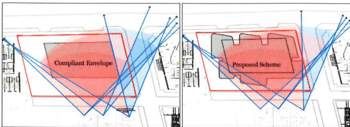
Figure 23 | View impact comparison between an ADG compliant envelope and the proposed envelope (indicative levels 8-17 of 90-102 Regent Street). Red illustrates view impact. Blue illustrates retained view corridor (Source: Applicant's RTS)
