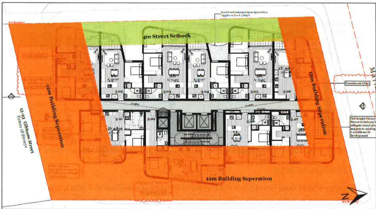
Figure 27 | Floorplan of levels 8 to 16 of the proposed tower overlaid with the ADG and SSP SEPP setback controls (Source: Architectural Plans)
