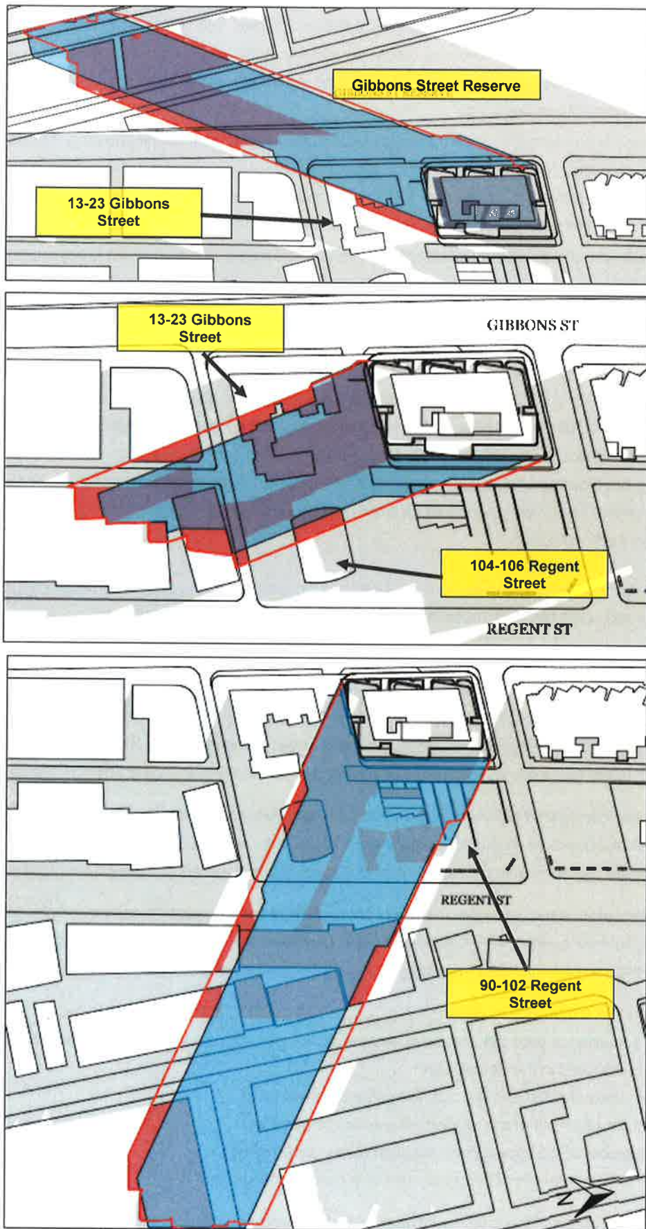
Figure 19 | Midwinter shadow diagrams (top: 9 am; middle: midday; bottom: 3 pm). Blue = shadow impact of a complying scheme, red = additional shadow from proposed development (Base source: Architectural Plans)
