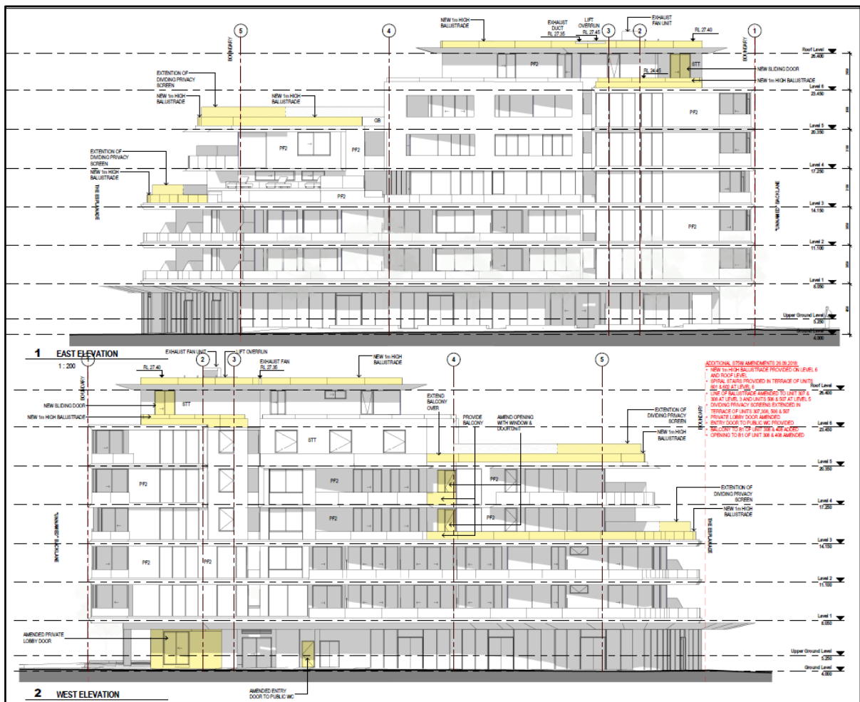
Figure 7 | Original proposed modifications to the East Elevation (top) and West Elevation (bottom) (Source: Applicant's Application)
