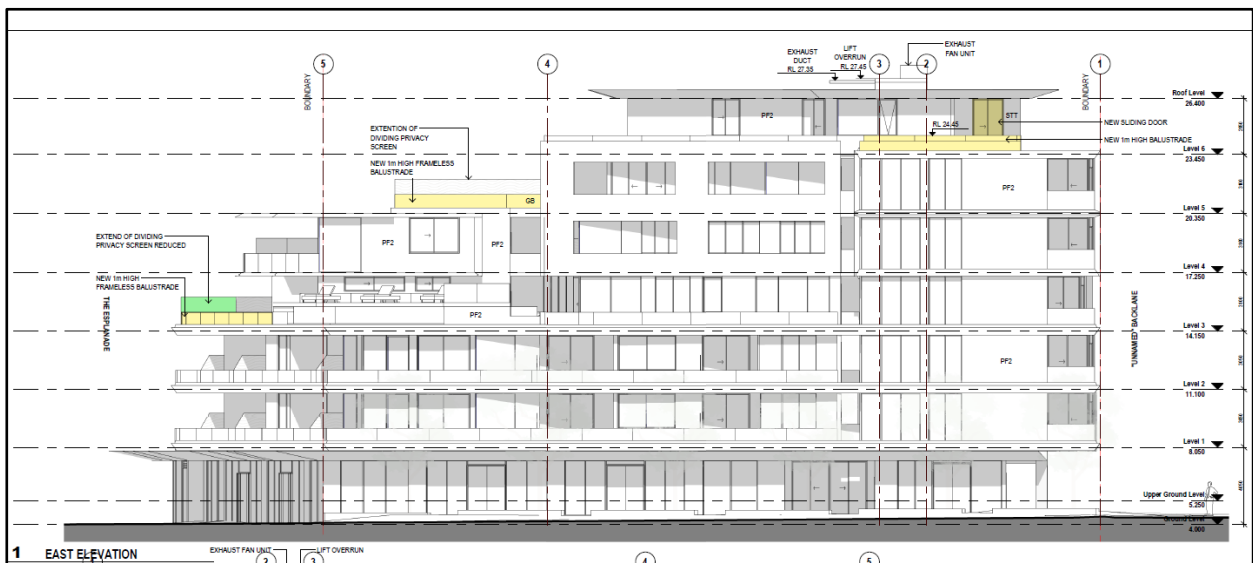
Figure 11 | East elevation with revisions to the Level 3 privacy screen shown in green (Source: RtS)
