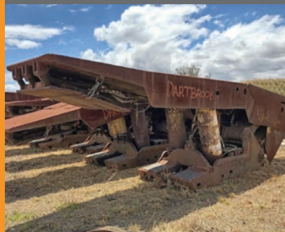
Roof support sections in storage
