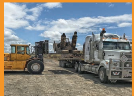
Loading dismantled longwall section to move offsite
