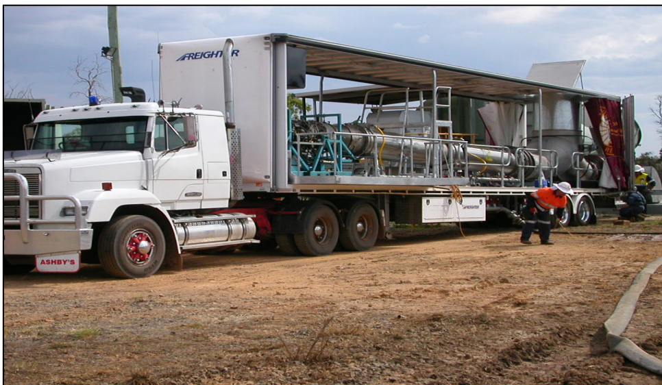
Figure 33: GAG engine set up for transportation and use
