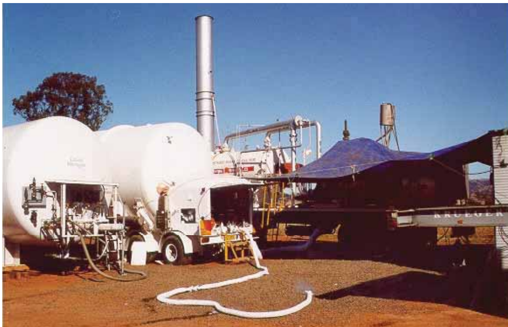
Figure 2.3 Mineshield inertisation unit on mine site
