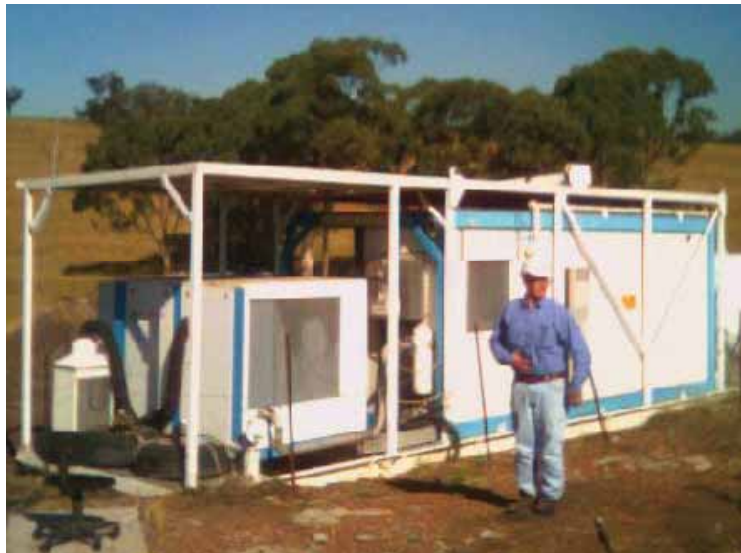
Figure 2.18 Floxal membrane inertisation unit at mine site
