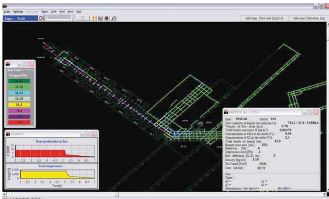
Figure 9.1 Oxygen distribution after 420 minutes.
