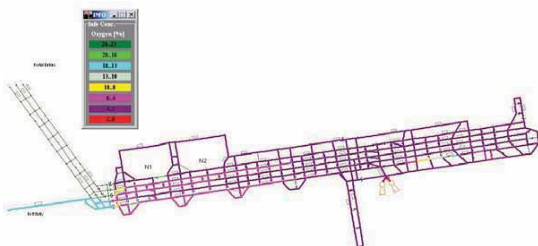
Figure 4.5 Oxygen distribution at 8.5 hours from VENTGRAPH simulation.
