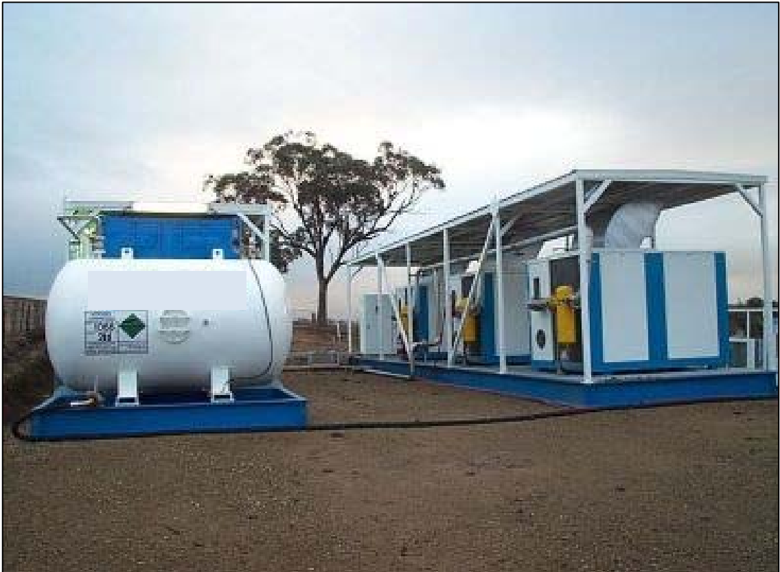
Figure 30: Membrane Separation Nitrogen Generator (Floxal)
