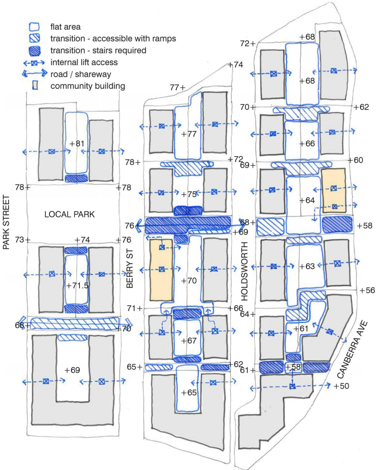
Fig 8.24 Required Site Levels
