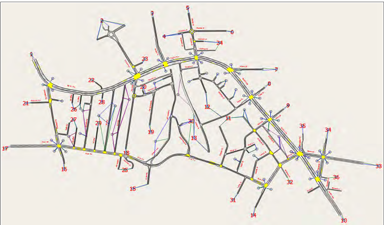
Figure 3: Aimsun model network structure
