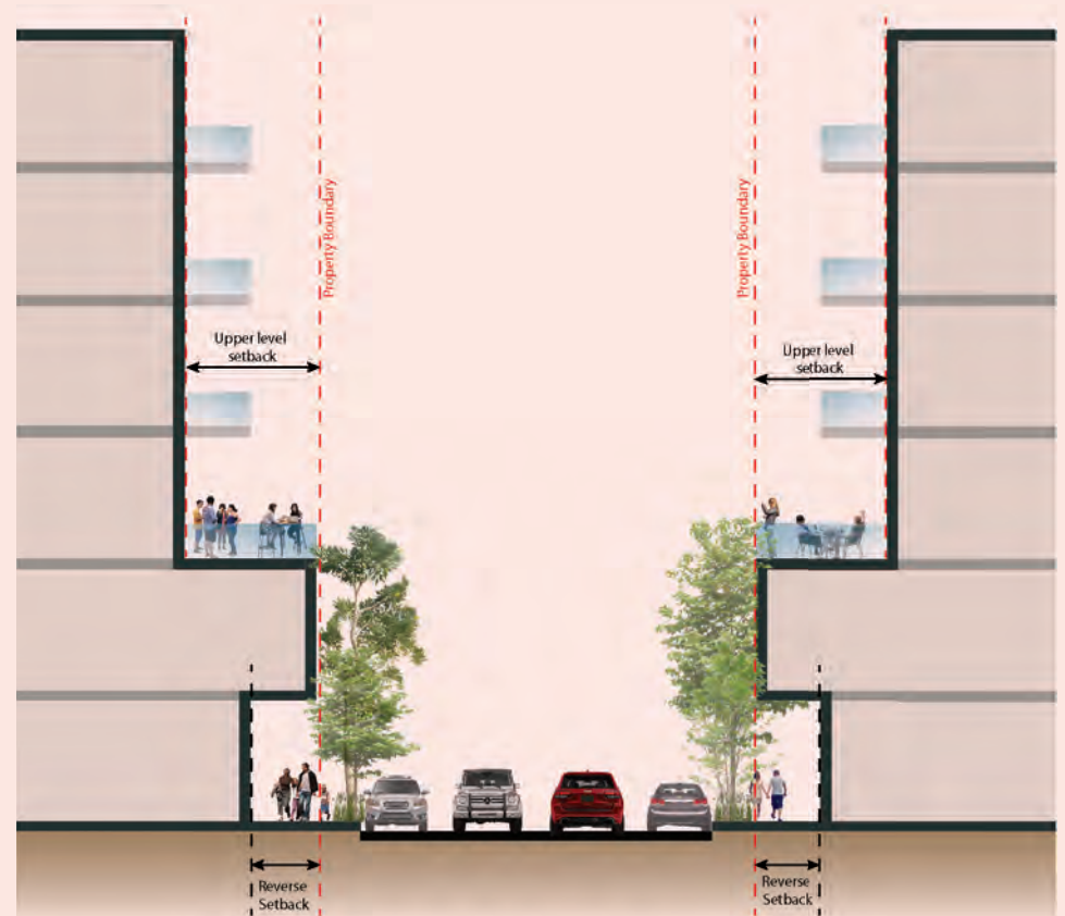
Figure 4: Ground floor setbacks for wider footpath
