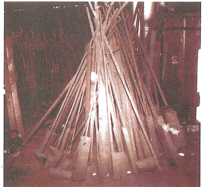
A very useful collection of Smithy tools. There is a large array of pick up tongs on the left side. These were used to pick up large forged pieces of steel from the hammers or after being cut to a predetermined size. In the centre area are heavy forge tools, formed swages and pads for forming corners and quickly reduce a slab of metal to a smaller size.
