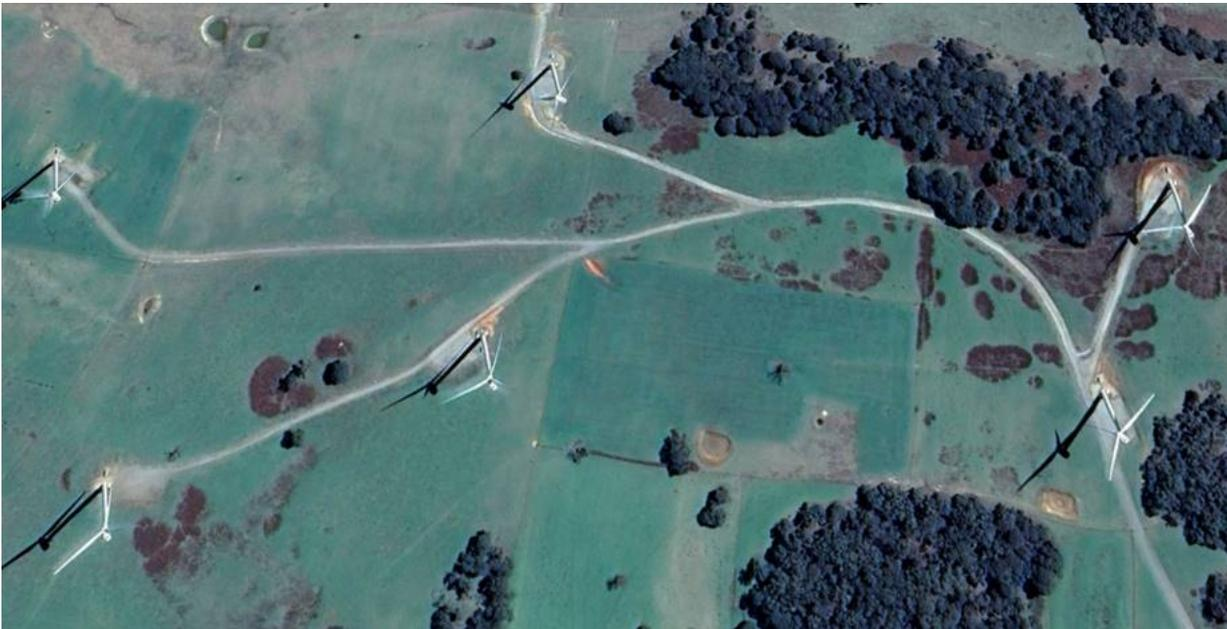
Note that even on relatively flat ground a larger construction footprint is required to build the roads and hardstands. This is then rehabilitated. Note also the underground cable runs.
