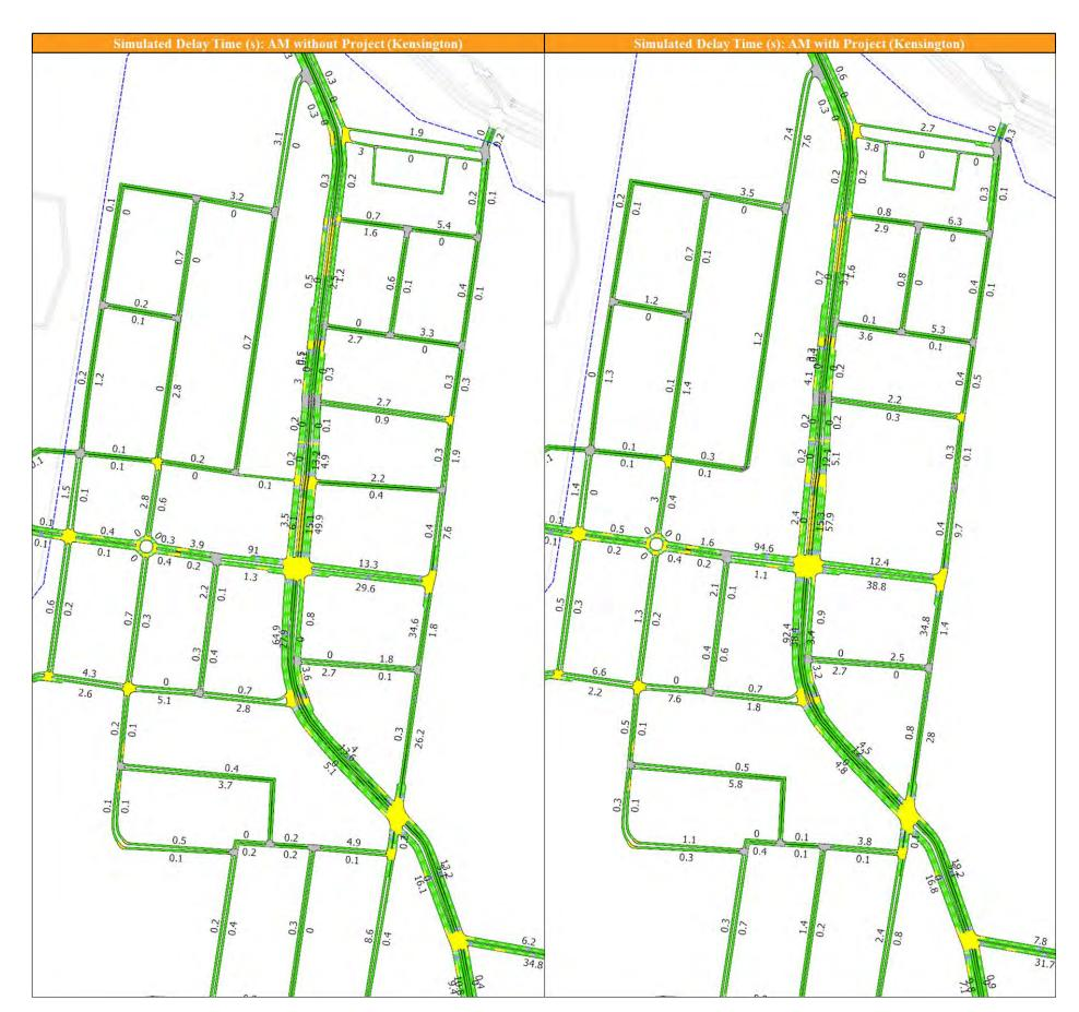
Figure 15: AM Simulated Delay Time Comparison (Kensington Town Centre)
