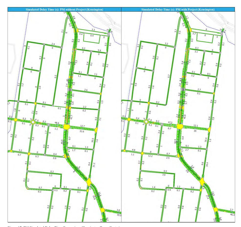
Figure 17: PM Simulated Delay Time Comparison (Kensington Town Centre)
