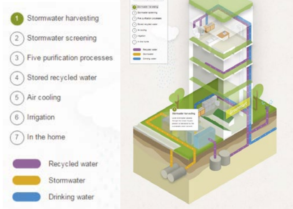
Figure 92: Diagram demonstrating the water recycling system at Green Square Source: Green Square Water
