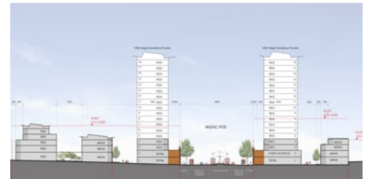
Figure 64: Section of Todman Square showing 18 storey building typology with four storey street wall and mews development at the rear. Source: Conybeare Morrison 2016
