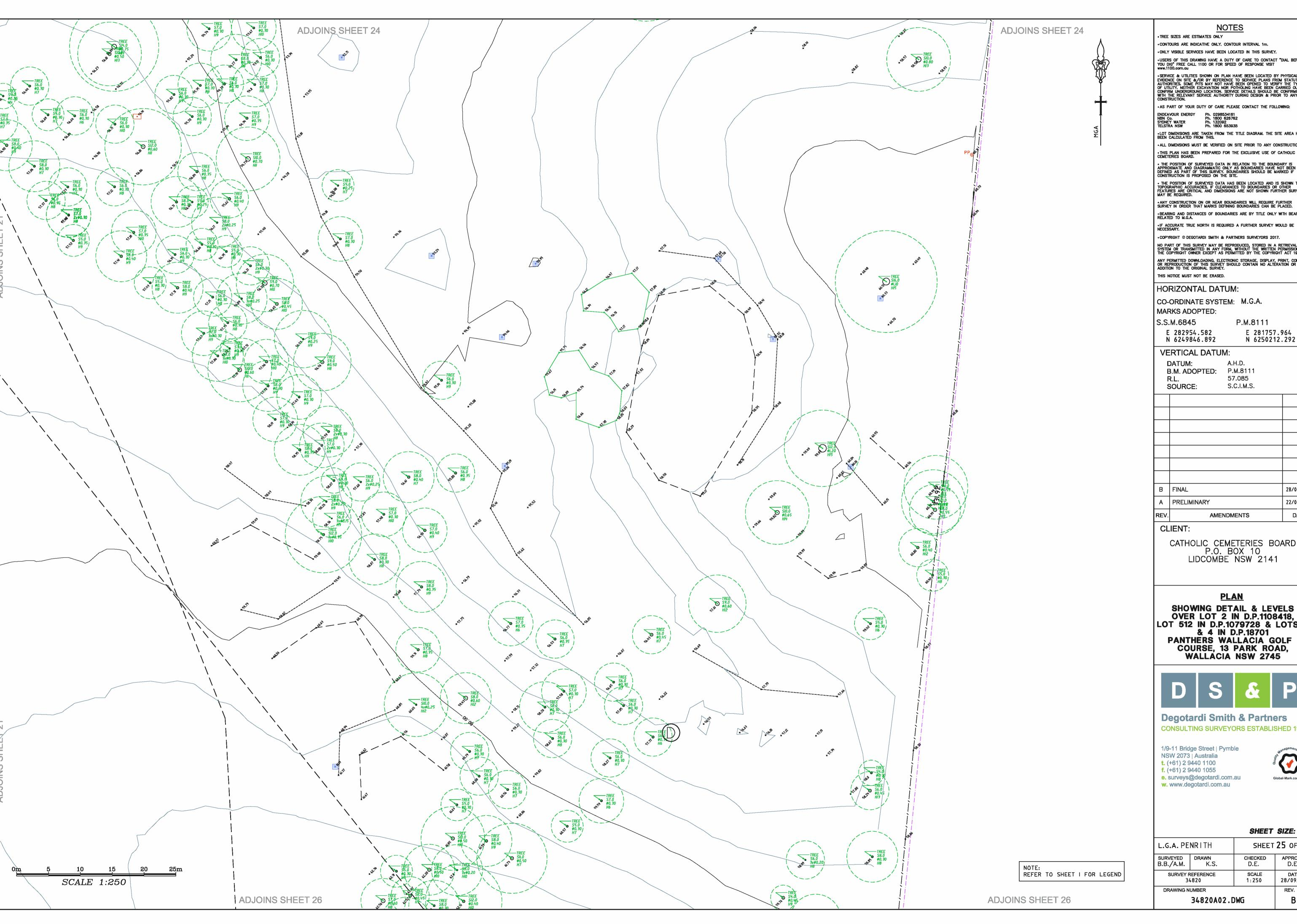
TREE SIZES ARE ESTIMATES ONLY • CONTOURS ARE INDICATIVE ONLY. CONTOUR INTERVAL 1m. ONLY VISIBLE SERVICES HAVE BEEN LOCATED IN THIS SURVEY.
