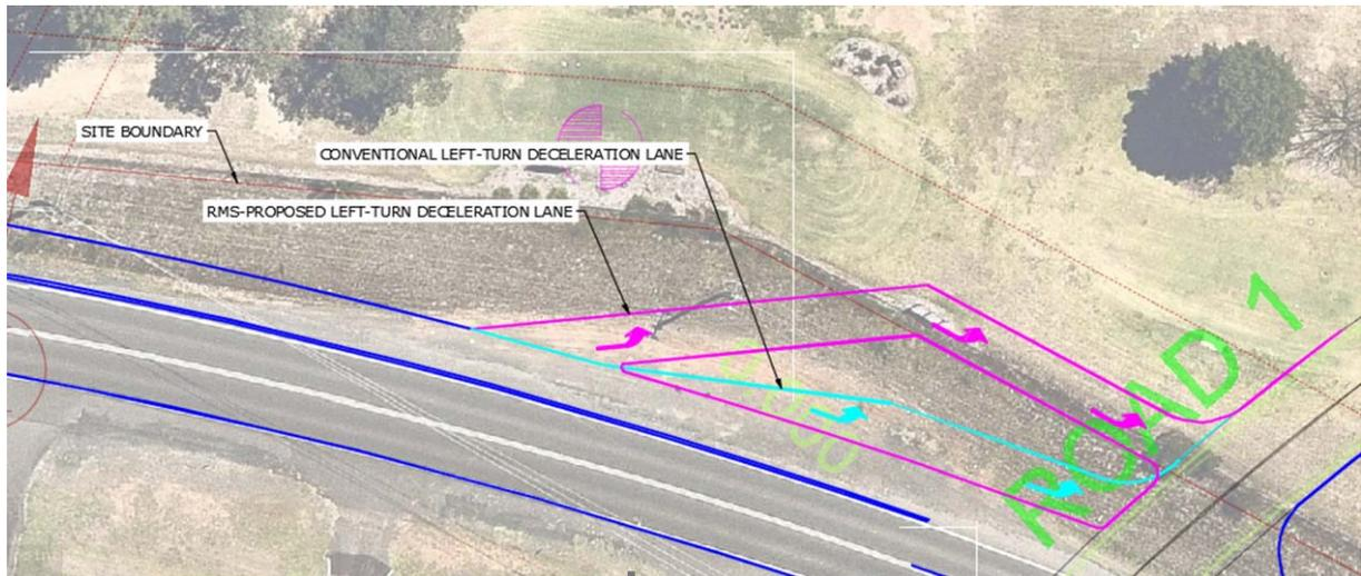
A deceleration lane by definition is an additional lane added to the through carriageway for safety and/or intersection capacity purposes. It is a means for the turning traffic to move into an adjacent lane to negotiate an intersection without interfering with the through traffic. This is as shown in light blue above.
