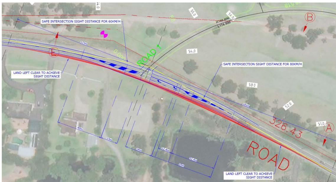
The proposed access point to and from Park Road, will be the main access point to the cemetery. The concept design shown above, has been developed showing the proposed Channelised T-junction (CHRs). Due to the road width available at the proposed access point, the road is to be widened to maintain traffic lanes in both direction and provide the CHR(s). The proposed priority intersection has been designed in accordance with the Austroads Guide to Road Design Part 4A (2017).
