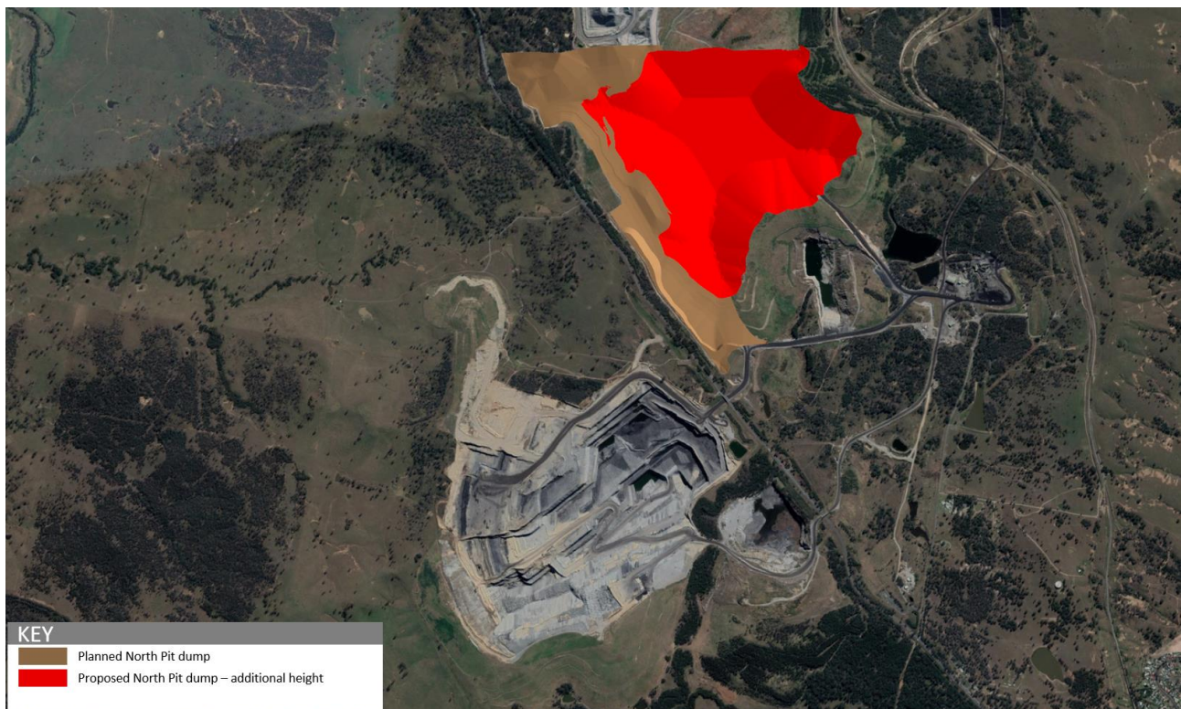
Figure 3 - Effect of Increasing Height of North Pit Dump
