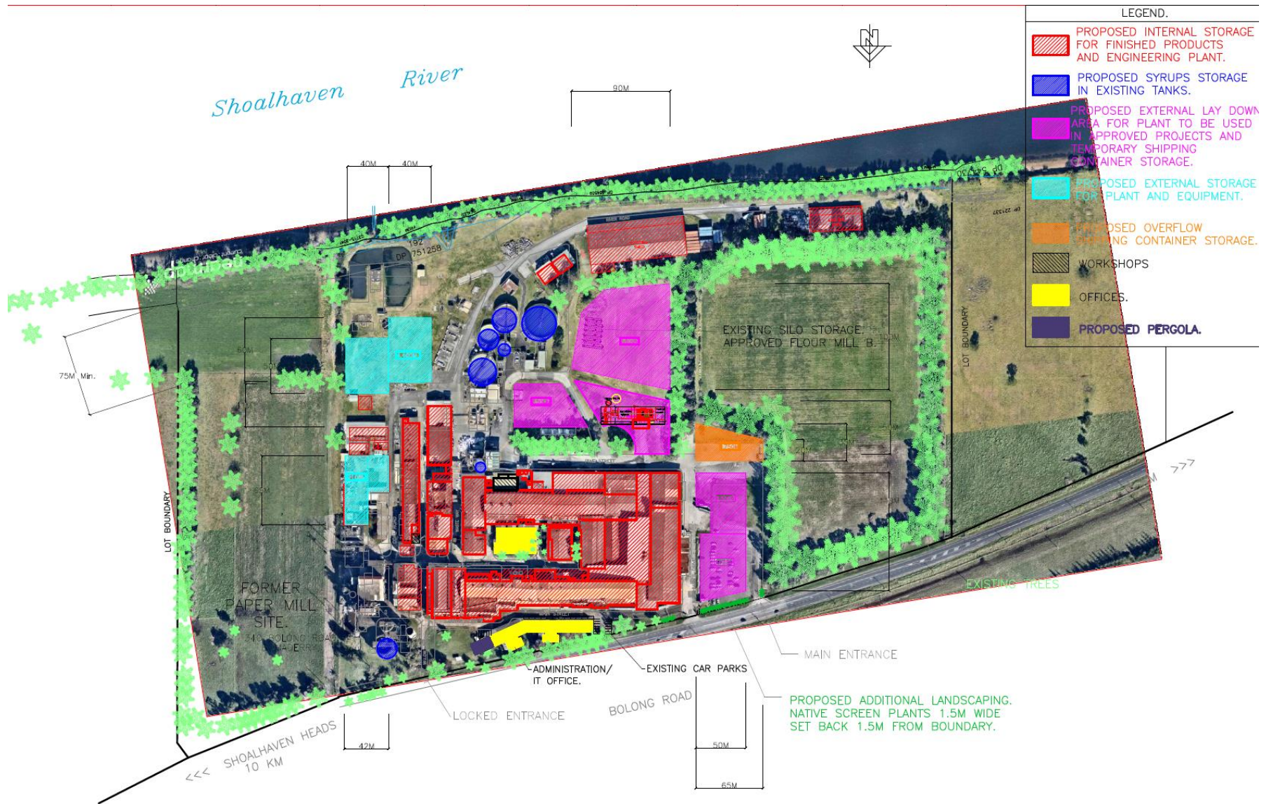
Storage Areas on Paper Mill Site
