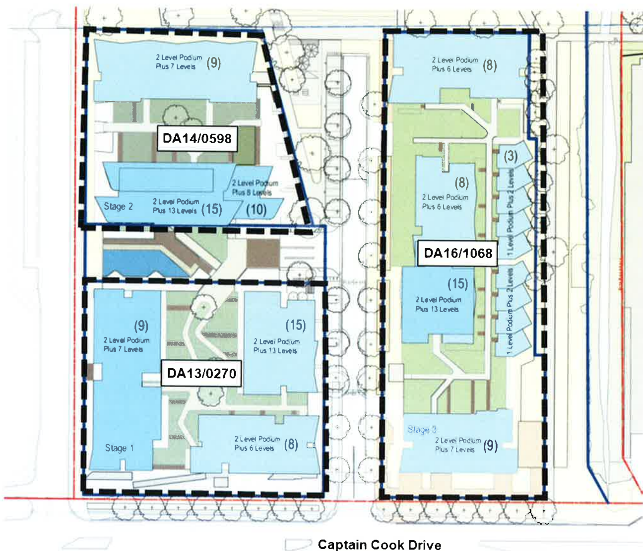
Figure 6: Stage 2 layout and building envelope heights (Base source: Proponent's PPR)
