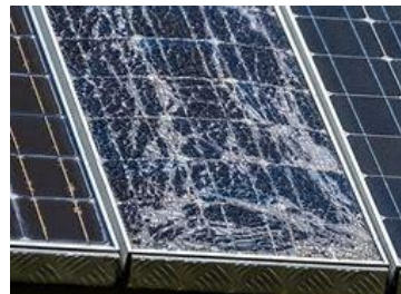
Examples of some types of PV panel deterioration
