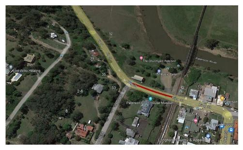
Paterson from the north and queued at the closed level crossing are totally concealed from further approaching traffic by a crest on a curve just 75 metres before the level crossing, trees along the left side approach to the crest and the location and height of the former church building on the left side of the crest. The height of this building is sufficient to block clear vision to the level crossing from the higher driving position of trucks.
