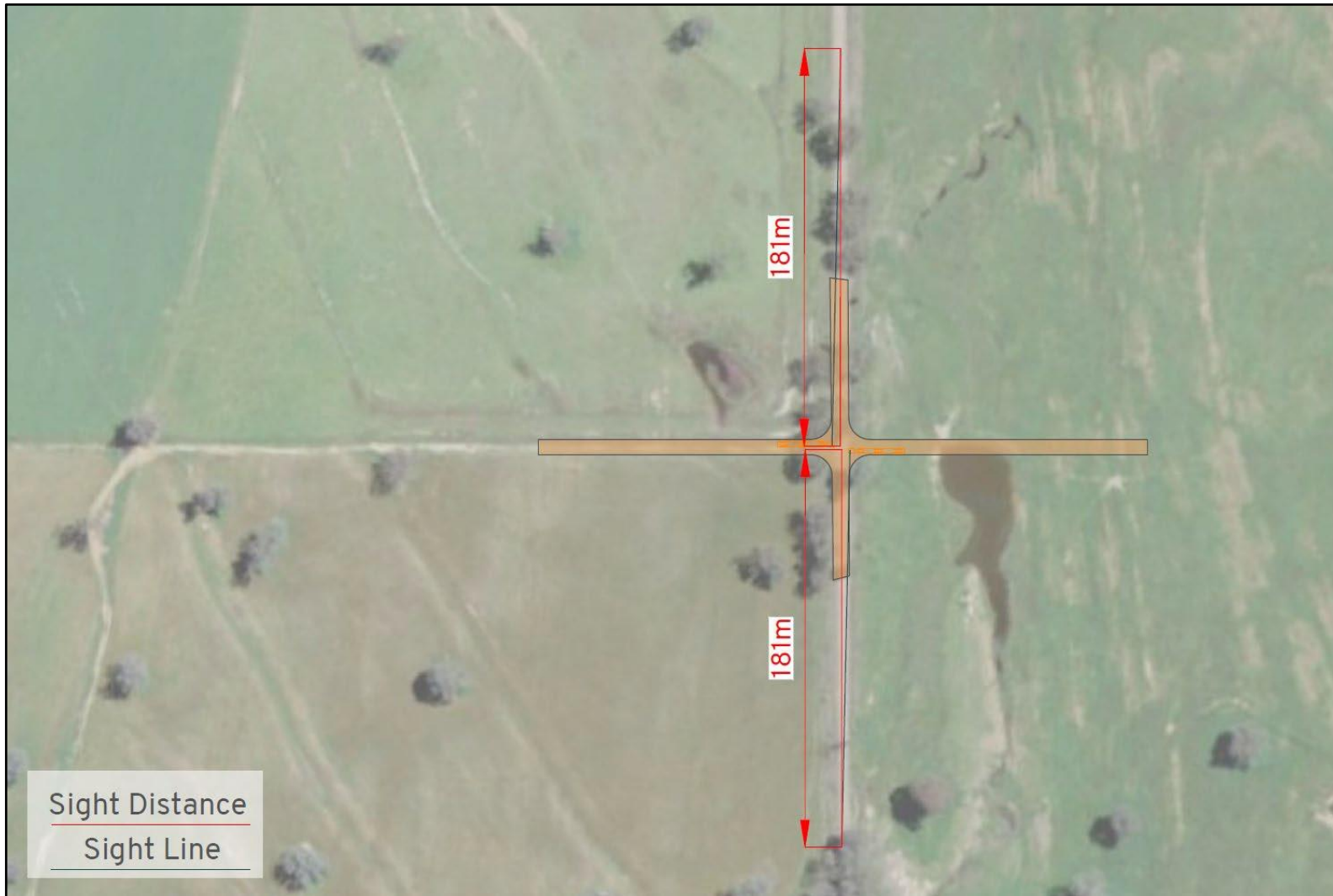
Figure 5 | Proposed access design for crossing points between east and western portions of the site
